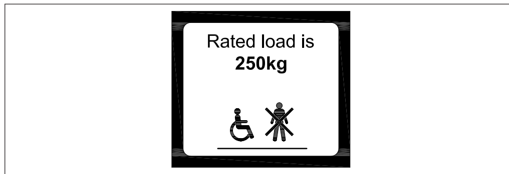
Figure 3 Typical load plate
