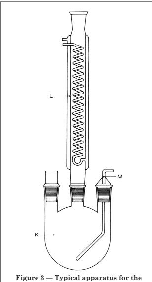
Figure 3 — Typical apparatus for the preparation of the reducing solution (8.3.7) used in the determination of content of sulphur compounds
