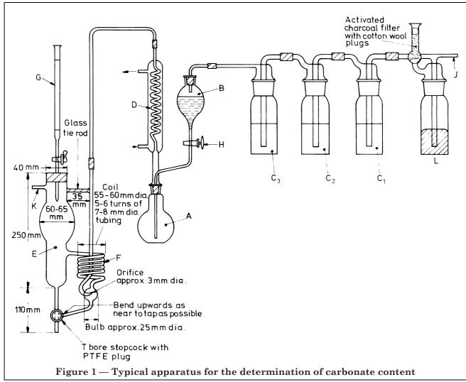
**5.5.3** *Determination.* Pass the nitrogen or the air (**5.3.6**) through the apparatus at a rate of about 5 bubbles per second for 10 min. Stop the current of gas and introduce the test portions and reagents into the apparatus as follows:
