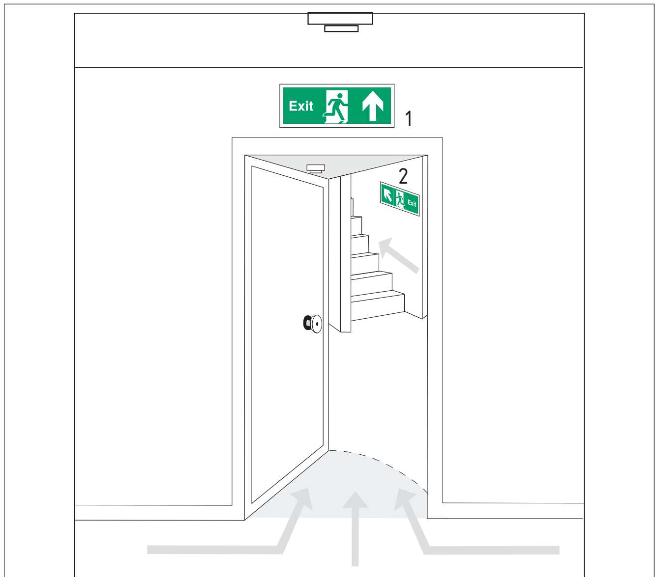
Figure A.8 Typical lobby entrance leading to left-handed ascent stairway showing the correct use of escape route sign(s) with supplementary text
