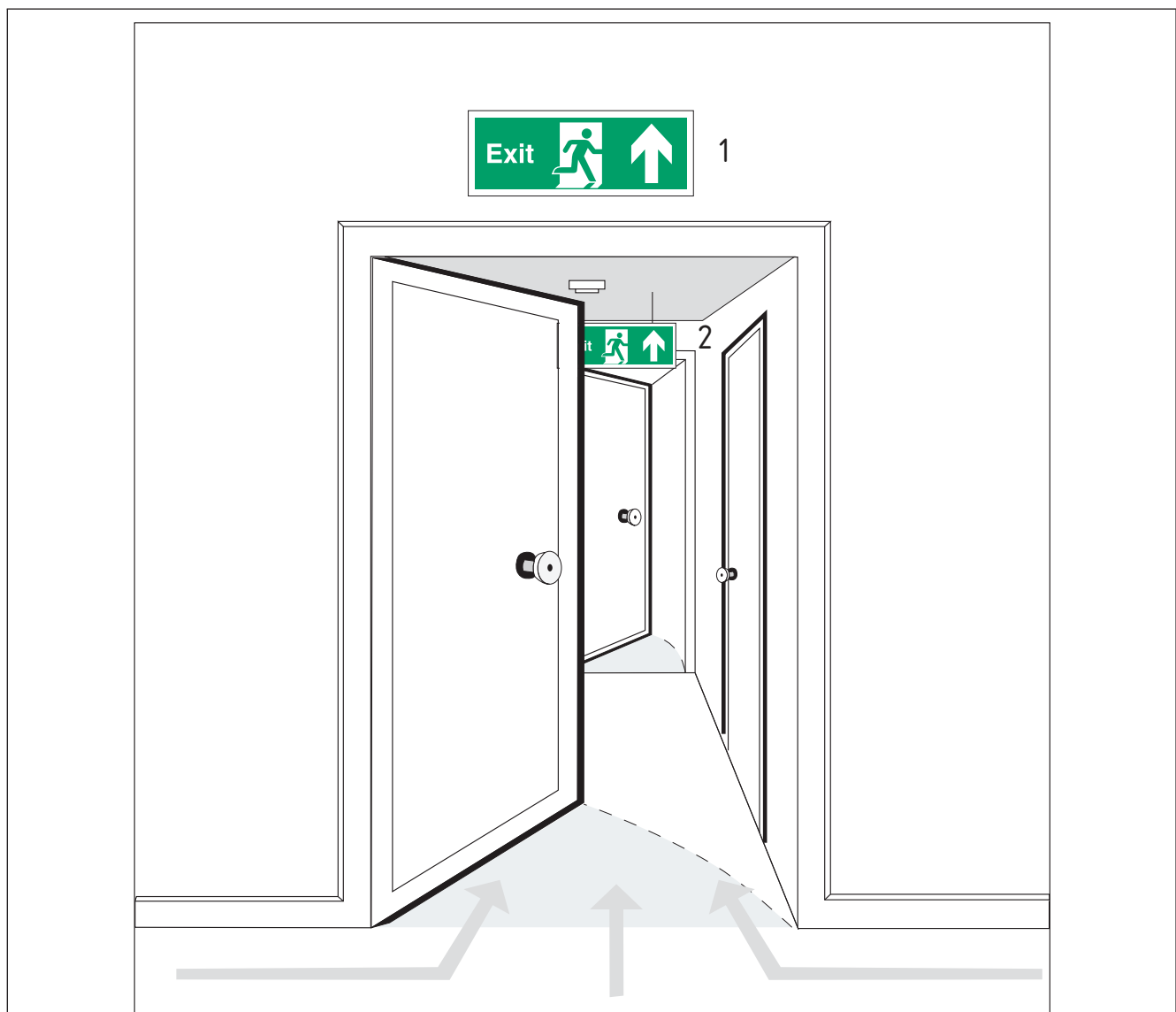
Figure A.1 Typical connecting corridor showing the correct use of escape route sign(s) with supplementary text
