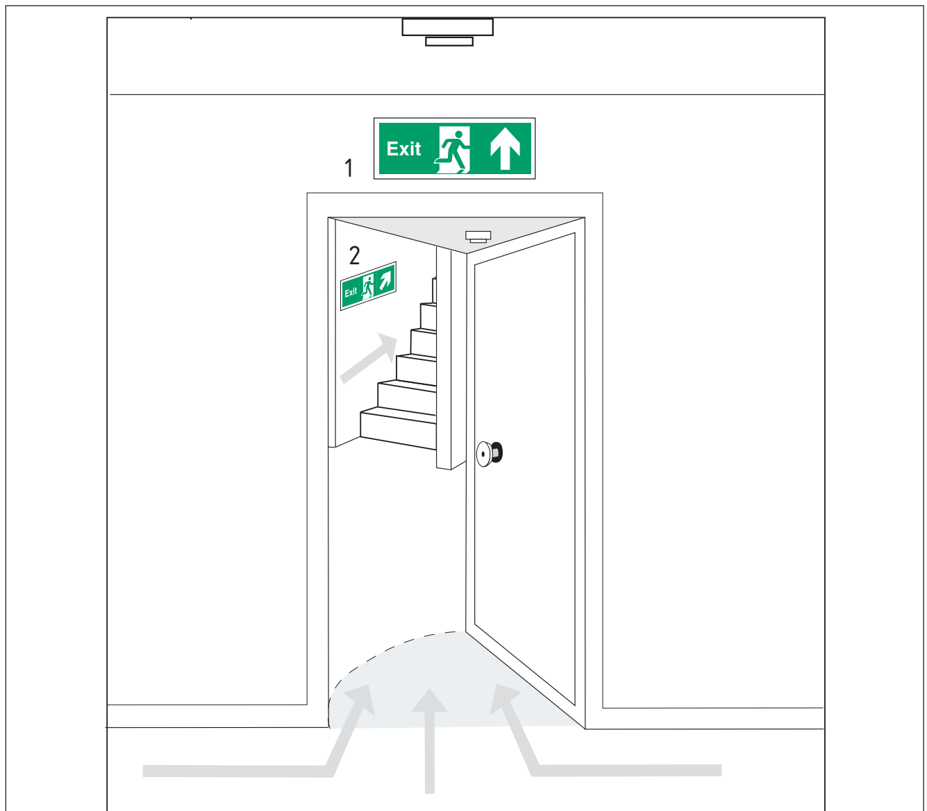
Figure A.9 Typical lobby entrance leading to right-handed ascent stairway showing the correct use of escape route sign(s) with supplementary text
