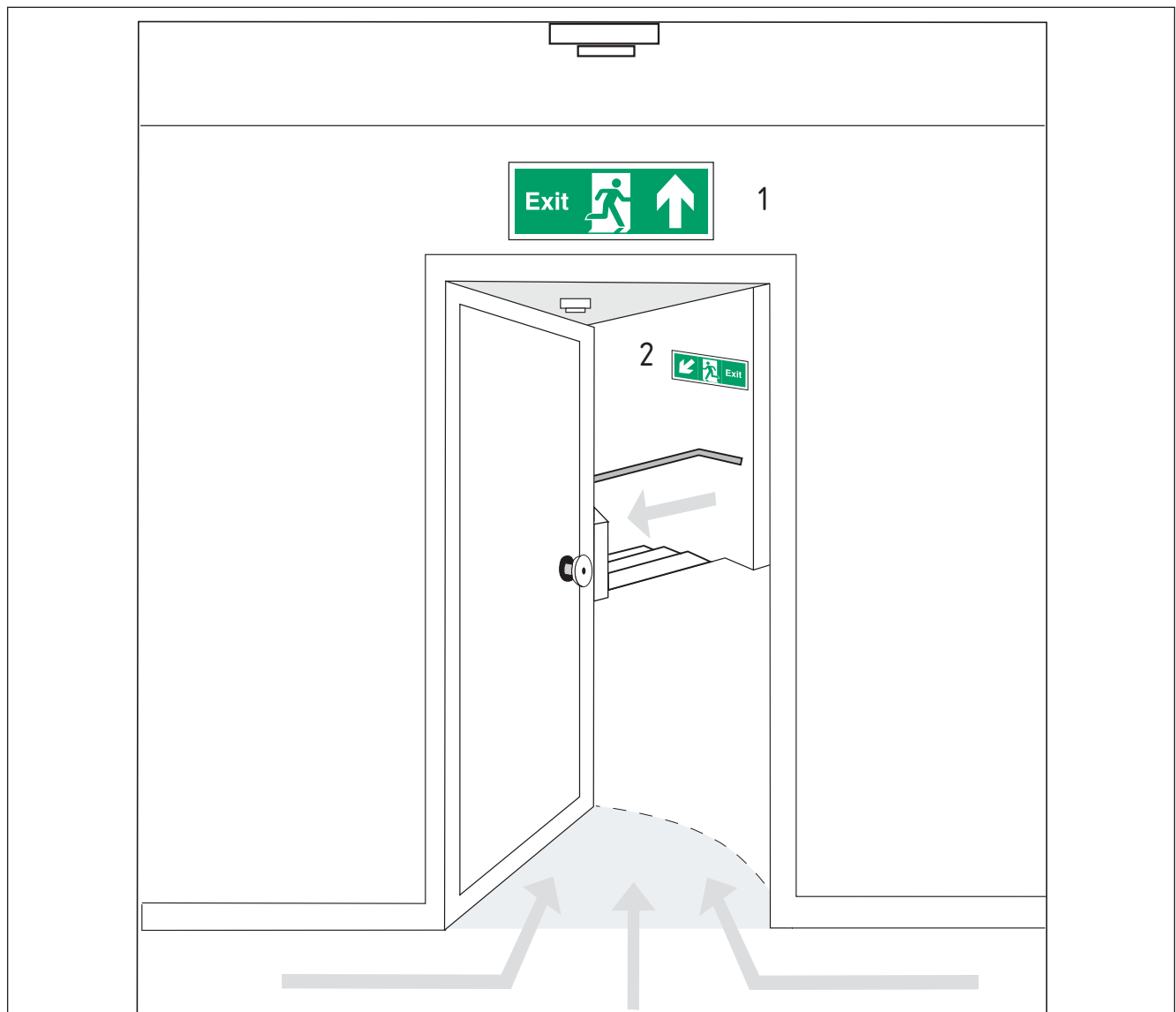
Figure A.6 Typical lobby entrance leading to left-handed descent stairway showing the correct use of escape route sign(s) with supplementary text
