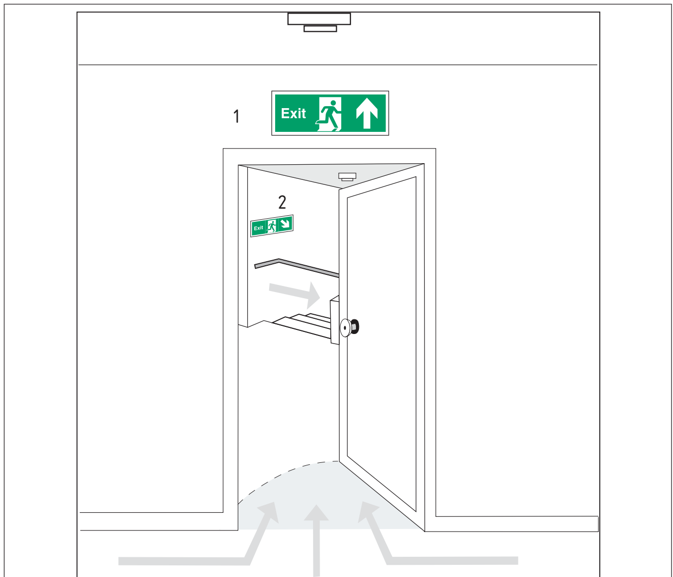
Figure A.7 Typical lobby entrance leading to right-handed descent stairway showing the correct use of escape route sign(s) with supplementary text
