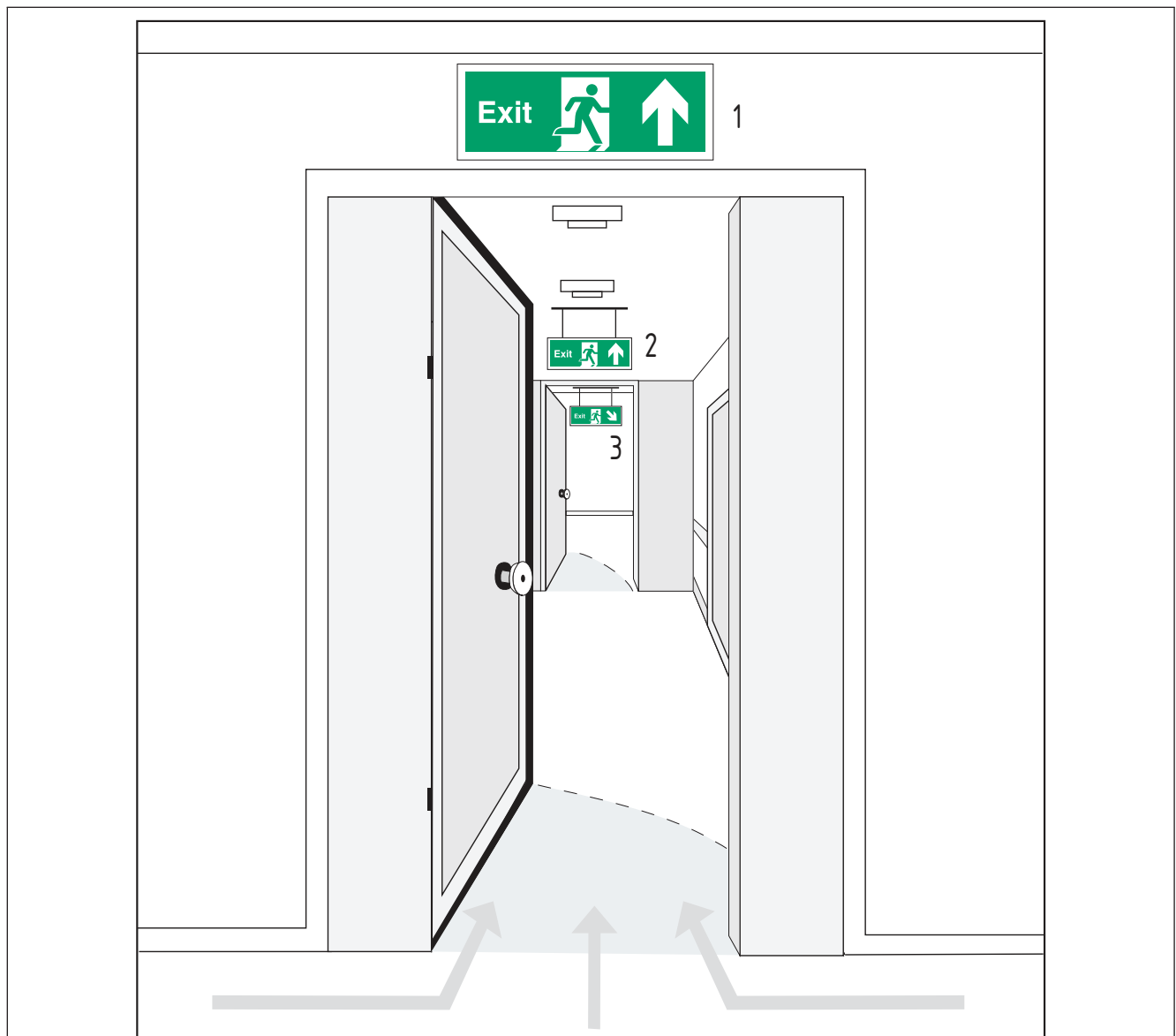
Figure A.11 Typical connecting corridor leading to descent stairway showing the correct use of escape route sign(s) and supplementary text
