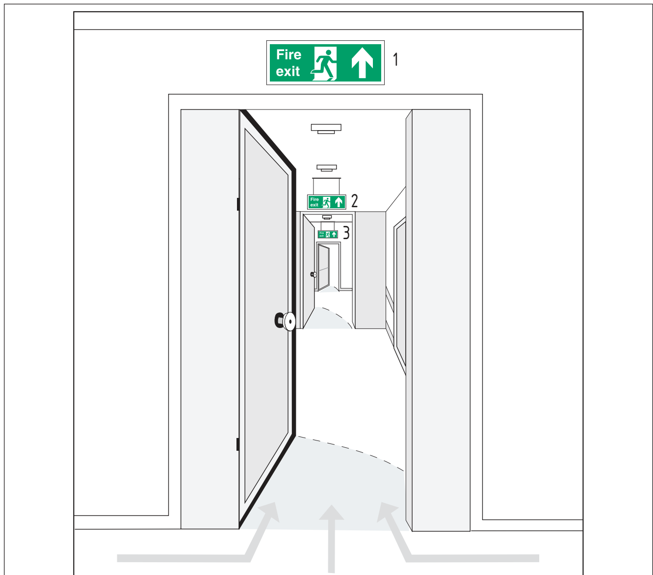
Figure A.10 Typical connecting corridor(s) to final fire exit showing the correct use of escape route sign(s) with supplementary text
