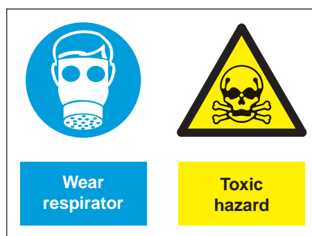
Figure 8 — Use of signs to convey more than one safety message with the inclusion of supplementary text signs
