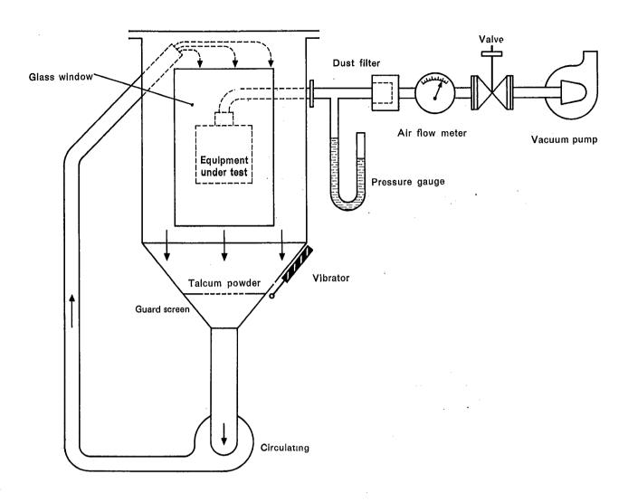
Fig. 2. — Equipment to prove protection against dust.
