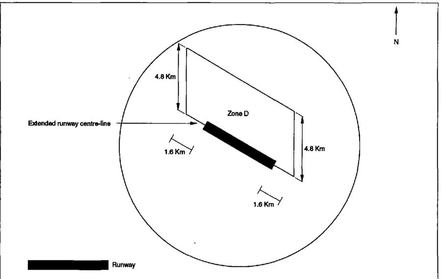
NOTE 1 Zone D is to the north of the runway. The northern boundary of zone D is 4.8 km from the runway centre-line, parallel to the centre-line. The eastern and western boundaries of zone D extend northwards from the runway centre-line produced 1.6 km from either end of the runway.
