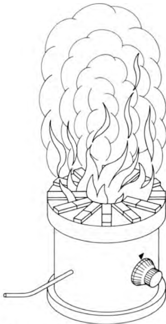
Figure 4 — Arrangement of beechwood sticks for test fire TF 2
