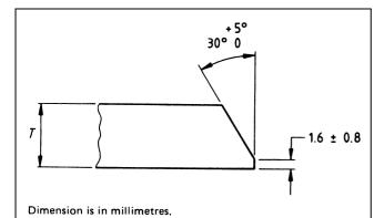
Figure 3 — Typical bevel for shell wall thicknesses (t) 22 mm or less for pipeline applications
