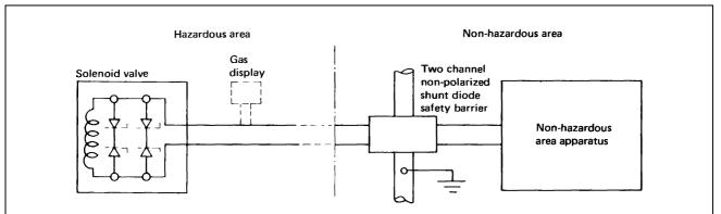
NOTE Compatibility of the two units is not readily demonstrated because of the complex characteristic of the partially suppressed solenoid. Hence system should be considered by a national authority.
