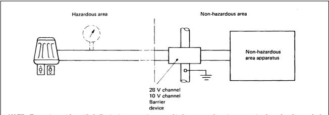
NOTE Transmitter with certified effective input capacitance, and inductance, and maximum permitted supply volts matched to barrier with certified maximum fault voltage and permitted hazardous area parameters.
