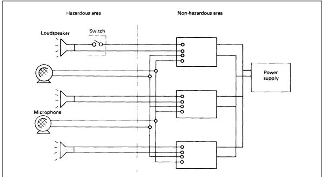
NOTE Where a specific combination is always used together, the whole may be certified to make best use of the system fault count. Switch to isolate a particular loudspeaker could be added as simple apparatus later (but see clause 8).
