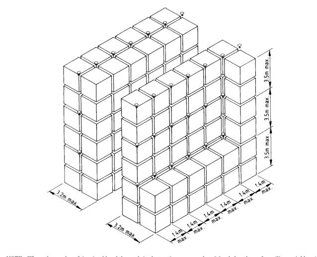
NOTE Where the number of tiers is odd and the goods in the top tier are more than 3.0 m below the roof or ceiling sprinklers (or are otherwise not protected by them), the rows of sprinklers shall be provided above each even-numbered tier, and above the top tier.
