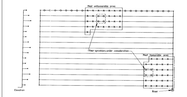
Figure 37 — Typical hydraulically most favourable/unfavourable locations of AMAO in an installation with gridded piping
