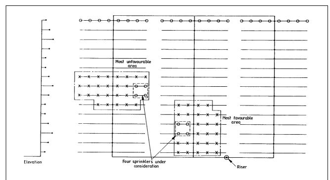
Figure 36 — Typical hydraulically most favourable/unfavourable locations of AMAO in an installation with looped distribution piping
