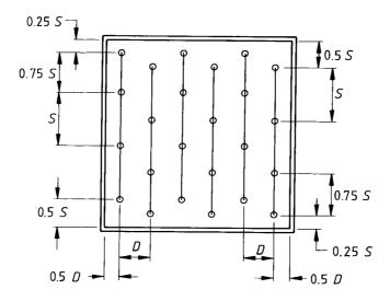
(b) Staggered layout for ordinary hazard systems where  $\boldsymbol{\mathcal{S}}$  is to exceed 4 m
