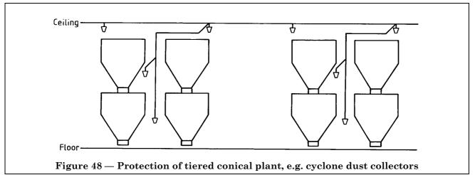
**26.7.3.3** Dust cyclones and dust collection chambers and boxes either inside the protected building, or outside and directly above any protected building with a combustible roof, shall be fitted with internal sprinklers.
