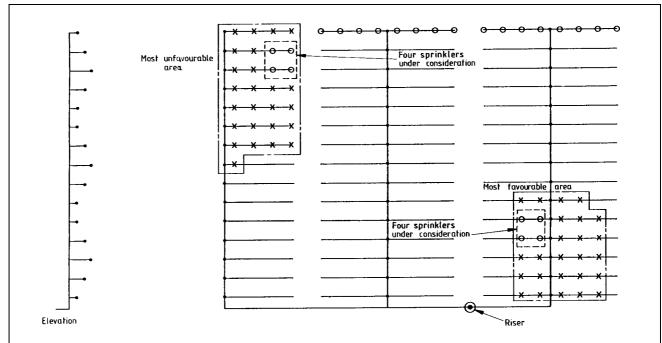
Figure~35 — Typical~hydraulically~most~favourable/unfavourable~locations~of~AMAO~in~an~installation~with~terminal~main~distribution~piping
