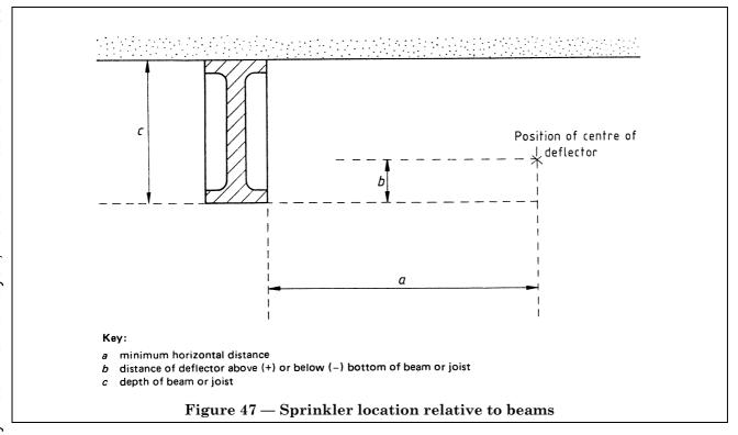
**26.5.3.2** Where the top flange of a girder is more than 200 mm nominal width sprinklers shall be positioned not less than 1.2 m from the side of the girder (viewed in plan).
