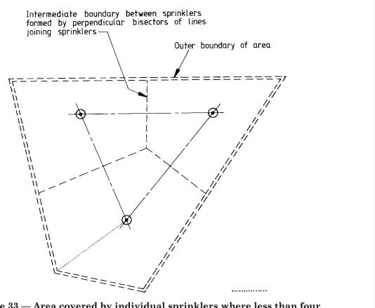
Figure 33 — Area covered by individual sprinklers where less than four sprinklers are in open communication
