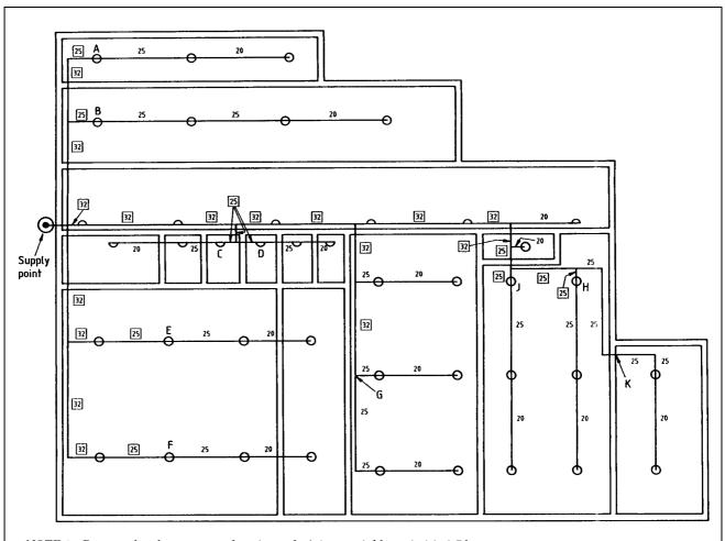
NOTE 1 Pressure loss between supply point and: A (two sprinkler point) is 0.7 bar
