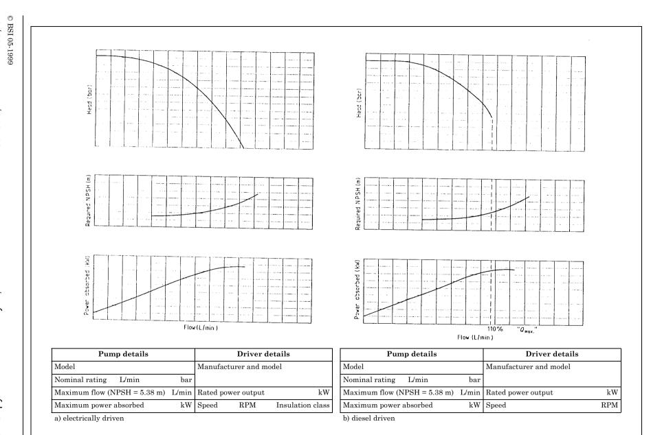
Figure 5 — Typical pump data sheet
