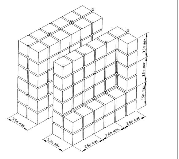
NOTE Where the number of tiers is odd and the goods in the top tier are more than 3.0 m below the roof or ceiling sprinklers (or are otherwise not protected by them), the rows of sprinklers shall be provided above each even-numbered tier, and above the top tier.
