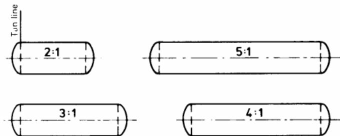
In calculating volumes of vessels "ellipsoidal" values from Table 4 are used for inside crown radii and inside knuckle radii of domed ends.
