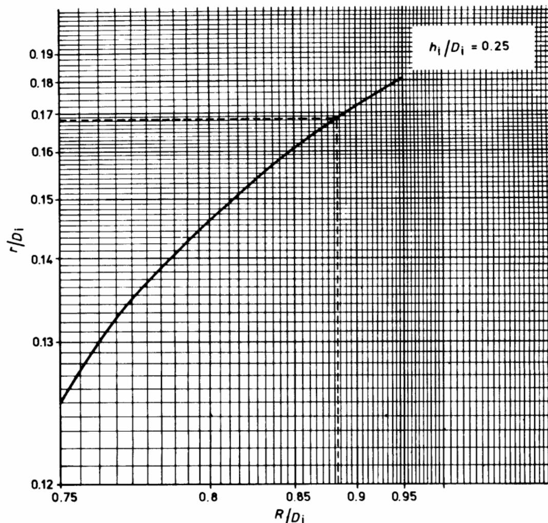
Graph for determining the appropriate values of  $R$  and  $r$  to give  $h_i/D_i = 0.25$
