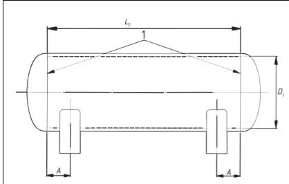
NOTE The minimum vessel length  $L_{\rm t}$  which will permit this location for the supports is 1 000 mm.
