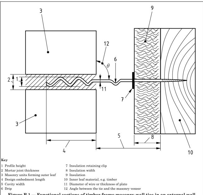
$\begin{array}{c} \textbf{Figure B.1-Functional sections of timber frame-masonry wall ties in an external wall} \\ \textbf{construction} \end{array}$
