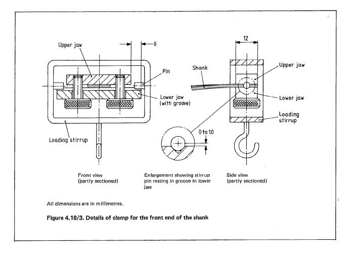
which hold the rear clamp in position. Position the dial gauge so that its shaft is vertical and in line with the centre of the top face of the loading stirrup. Lower the dial gauge until the large pointer has rotated at least twice, i.e. 2 mm of movement and clamp by tightening G.
