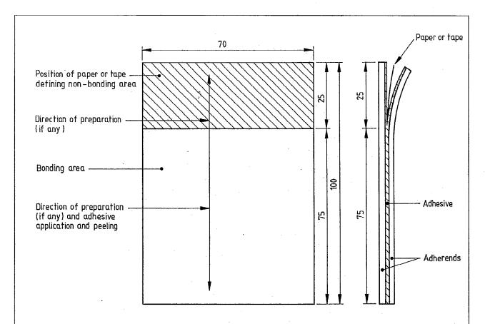
(a) Plan view of test assembly
