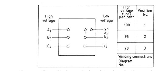
Figure 1 — Example of a terminal marking plate showing standard items of information to be provided and their arrangement
