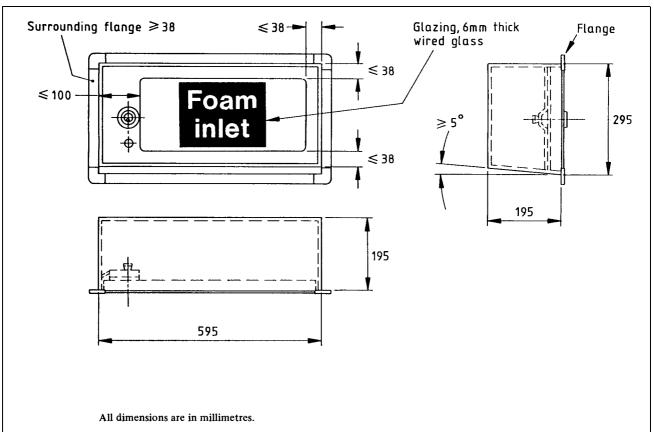
Figure 1 — Typical drawing of box for 2 foam inlets
