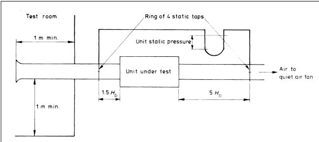
Figure 5 — Arrangement of equipment for generated noise test; noise radiated, in direction of inlet
