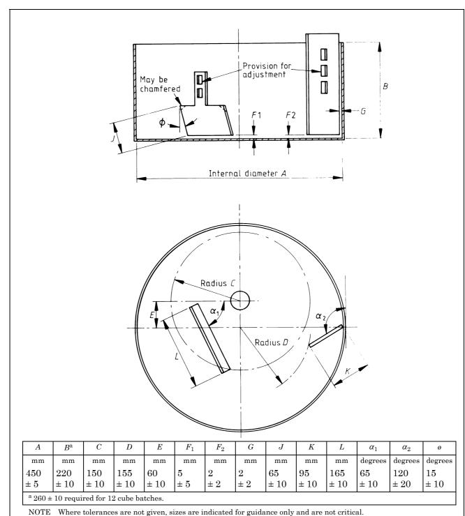
Figure 1 — Typical rotating pan concrete mixer
