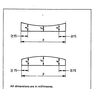
Figure 2. Thickness across a transverse cross section of a wide flat
