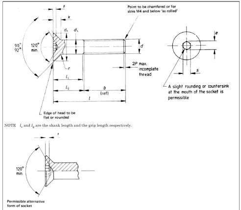
$NOTE \quad For broached sockets which are at the maximum limit of size, the overcut resulting from drilling shall not exceed 20 \% of the length of any flat of the socket.$
