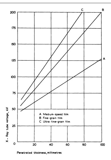
NOTE The thickness in question is the total thickness penetrated. This may include a backing ring, excess weld metal, and, in the case of double wall methods, an additional wall thickness. The radiographic sensitivity should be calculated with respect to this total thickness penetrated. It should be recognised, however, that the sensitivity of flaw detection is impaired by superimposed metal thickness.
