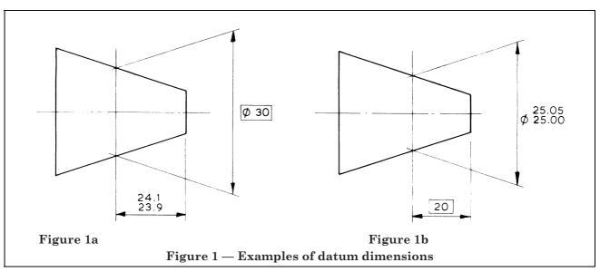
When converting datum dimensions from one system of units to the other, care should be taken to ensure that the errors of this conversion do not add to those arising from the conversion of the associated toleranced dimensions. Rules 7 to 11 help to avoid such accumulation of errors.
