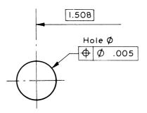
The above method of dimensioning, recommended in BS 308-3, means that the true position of a certain feature (the hole) is located by a dimension 1.508 inches (True Position) and the axis of the feature is allowed to depart from that true position providing it lies within a 0.005 inch diameter cylindrical tolerance zone, centred on the true position.
