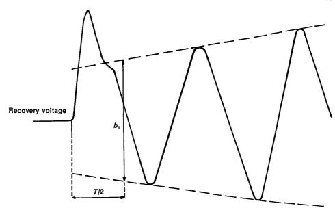
T =duration of first power-frequency cycle following initiation of test.
