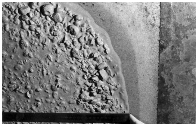
(b) Lack of cohesion in the concrete has resulted in grout segregation round the perimeter of the sample
