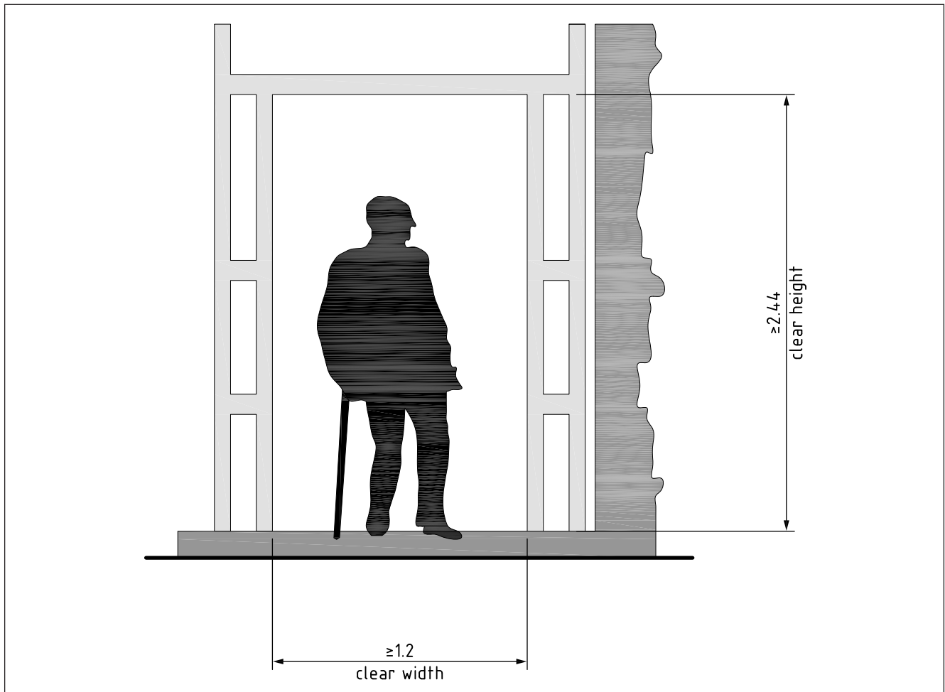
Figure 15 Minimum clear height and width for walk through end frames on the highway for the passage of the general public
