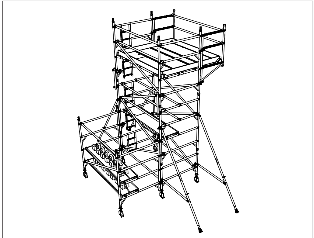
Figure 1 Example of a cantilever tower scaffold
