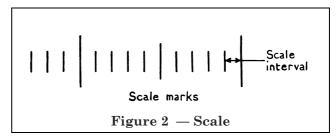
On multi-range scales, at least every tenth interval shall be numbered and the value of each scale interval shall be clearly marked within the scale area using a suitable code to identify scale and scale interval values.
