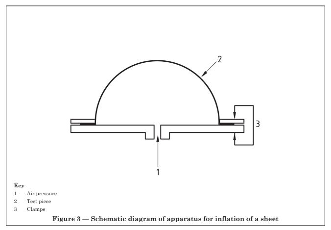
A flat rubber sheet is inflated through a circular clamp as shown in Figure 3. Near the apex of the sheet the rubber is in a state of equibiaxial strain. Only points within about  $10^{\circ}$  of the apex conform closely to the equibiaxial strain state, so measurements should be taken within this region.
