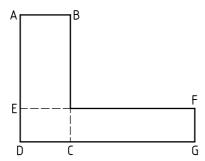
Thus, with the angle shown in the sketch, the rectangles are ABCD and DEFG respectively. The tolerances on the thickness of the legs shall be calculated as for rectangles of widths AD and DG respectively.
