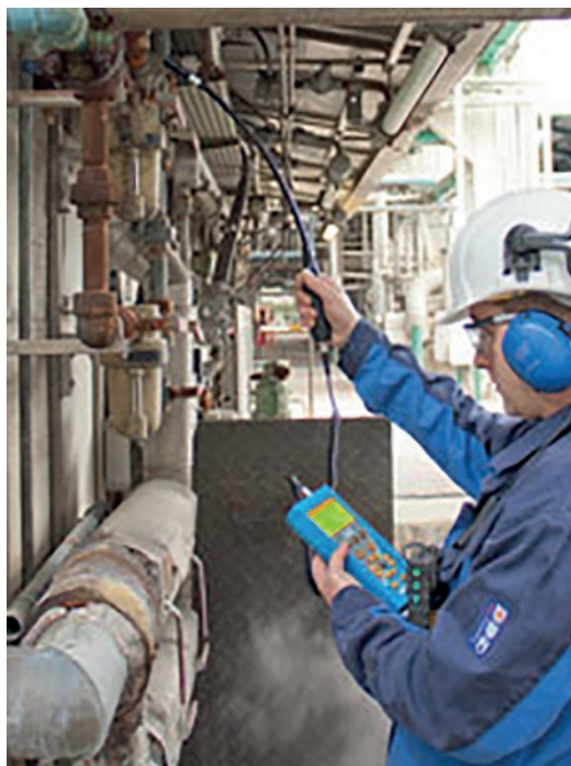
Figure 1 — Example of airborne ultrasound monitoring
