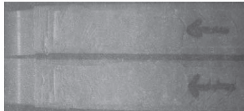
Figure 7 — Fracture surface of two halves of crack run-arrest specimen indicating the crack-arrest position
