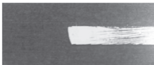
Figure C.1 — Straight-terminated crack front observed on crack-arrested specimen
