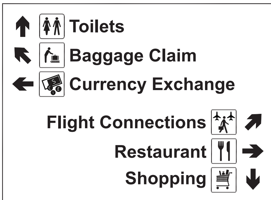
Figure 8 — Example of direction sign showing ranging of messages according to arrow direction and vertical stacking of messages
