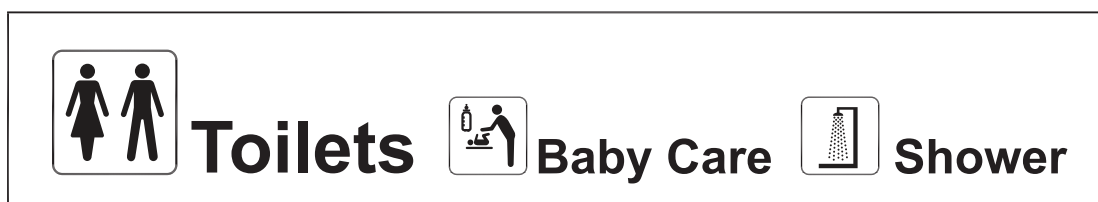
Figure 5 — Examples of location signs showing the prioritization of functionally related symbols with different graphical symbol sizes and text size
