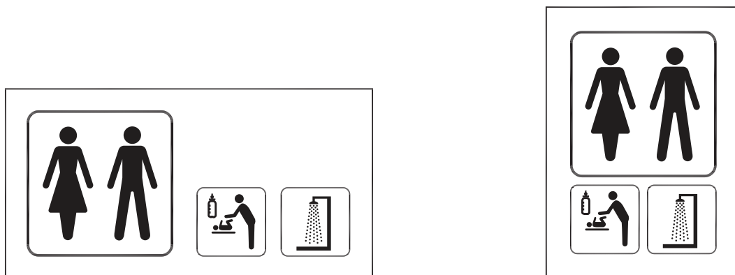
Figure 4 — Examples of location signs showing the prioritization of functionally related symbols with different graphical symbol size
