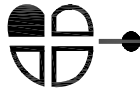
Figure B.7 — Example of a symbol that represents a signal coming from the heart
