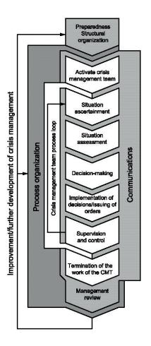
Figure 2 — Schematic work flow of a CMT
