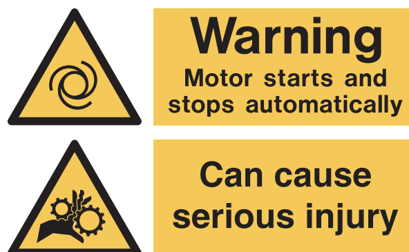
Figure 12 — Example of a combination sign consisting of ISO 7010-W018 with a graphical (hazard or risk consequence) pictorial panel supplementary sign and supplementary text supplementary signs
