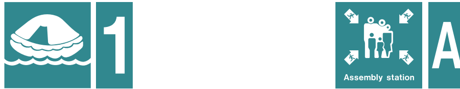
Figure 10 — Examples of combination signs using management information panel supplementary signs (with internal borders)
