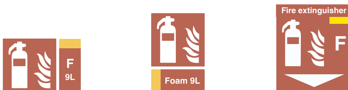
Figure 8 — Examples of combination safety signs using identification description panel supplementary signs (with and without internal borders)
