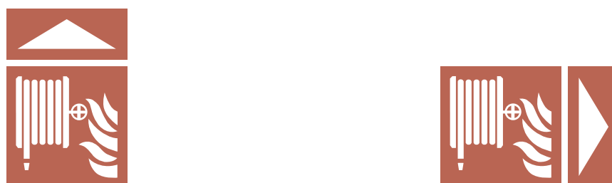
Figure 9 — ISO 7010-F002 example of combination signs using location indicator panel supplementary signs (with internal borders)
