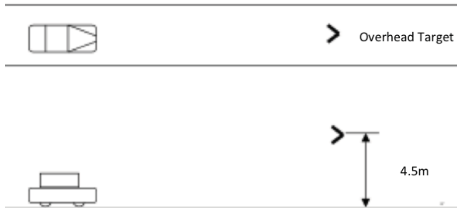
Figure 15 — Overhead target discrimination ability test
