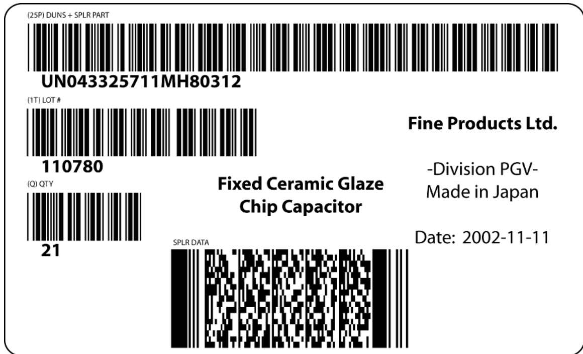
Figure 11 — Example of linear bar code symbols and PDF417 with DIs (not to scale)
