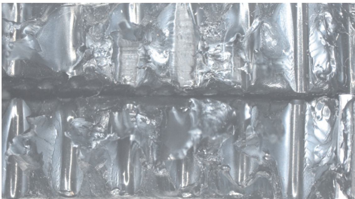
Figure 4 — Typical brittle fracture – side view
