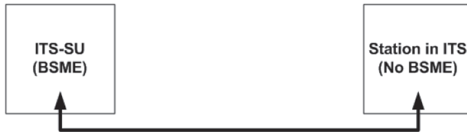
Figure 5 — BSME to ITS station unit (no BSME) communication without an external network (single-hop)
