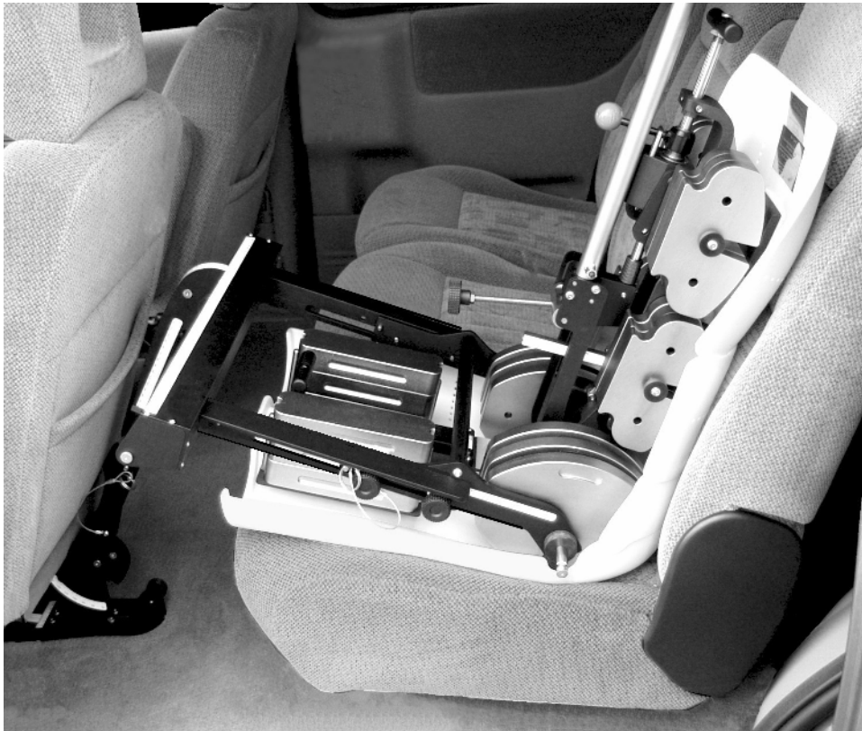
Figure 12 — H-point machine installed in rear outboard seat
