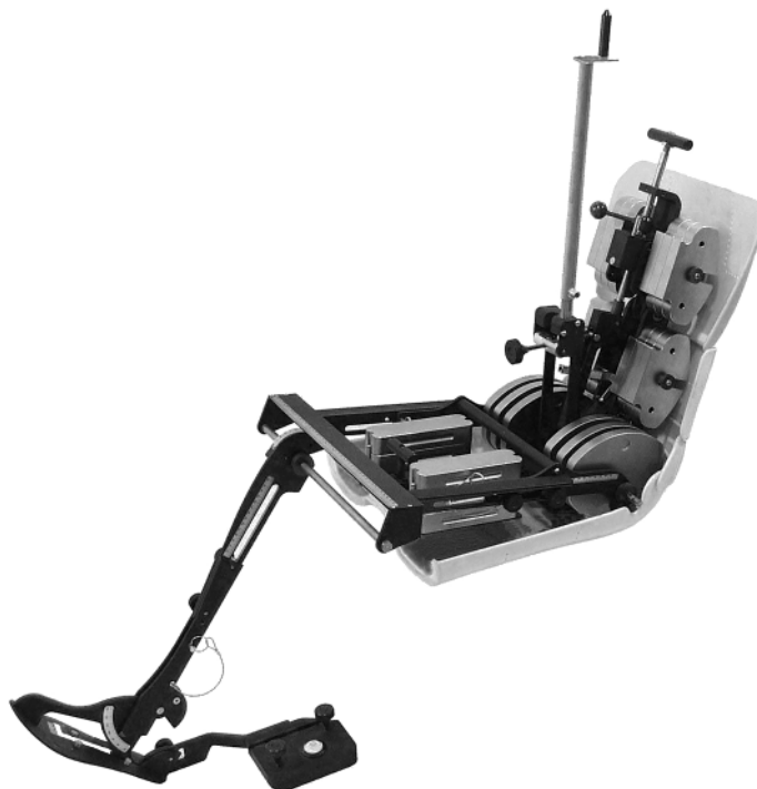
Figure 7 — Perspective view of HPM, including optional components
