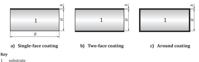
Figure 1 — Schematic of cross-section of test piece with different coating configurations
