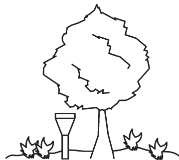
Figure 9 — Schematic showing criteria for precipitation for class 5 sites
