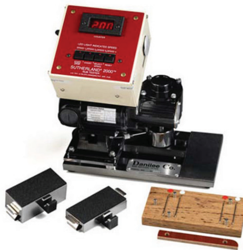
Figure A.1 — Test device described in ASTM D 5264, ASTM F 2497 and ASTM F 1571
