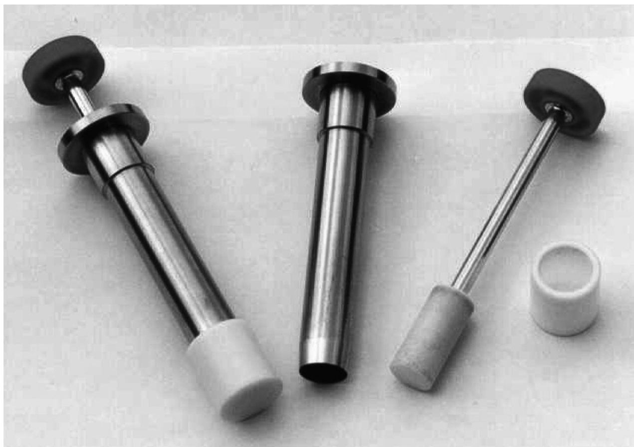
Figure 1 — Example of a core sampler made of metal with a PTFE syringe plug for sampling soils containing volatile organic compound (Inst. Berghof, Tübingen)
