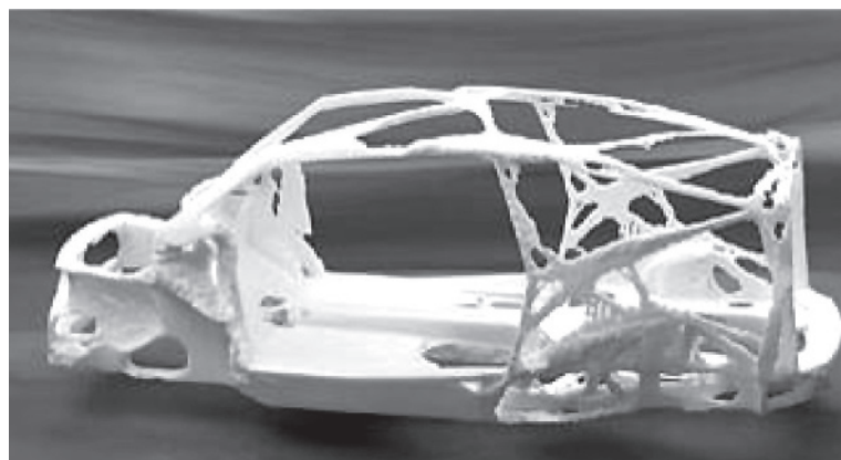
Figure 6 — Result of SKO optimization, an optimal frame in terms of stiffness and weight for the loads applied
