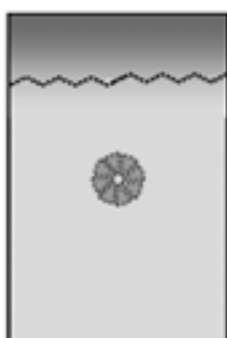
NDT indication: end crushing a
