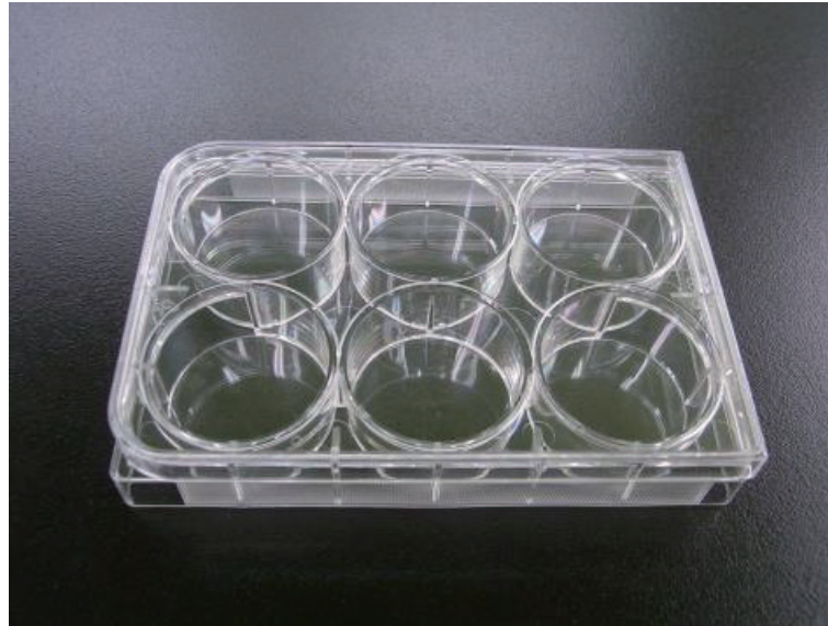
Figure 2 — 6 wells plastic plate for plaque assay
