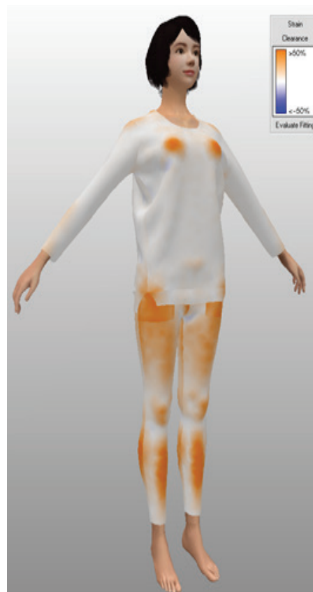
Figure 6 — Example of visualization of gap using pattern strain using colour scale
