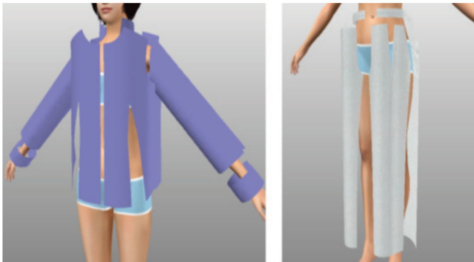
Figure 9 — Example of arrangement of virtual garment patterns
