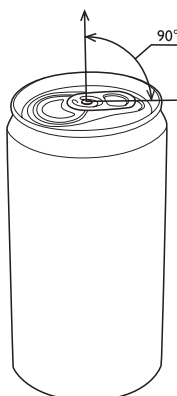
Figure B.7 — Illustration of mechanical tensile measurement
