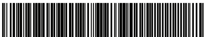
Figure B.3 — Code 128 encoding “25SUN043325711MH8031200000000001”
